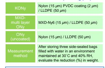
PVDC-coated nylon provides better moisture-proofing properties than ordinary nylon or MXD-multi layer nylon.
